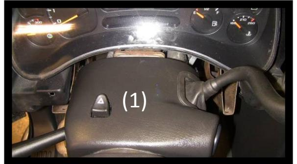
11. Using a 7mm socket; remove the plastic panel below the steering column.
