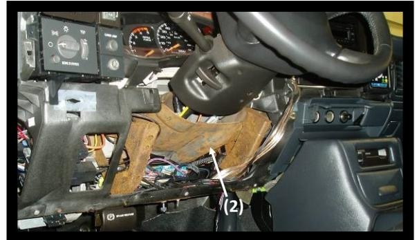
13. Unplug the factory shifter wiring harness. It is a black 2-pin plug.
