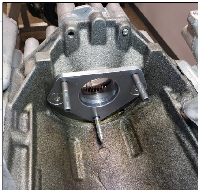
Figure 24: Engine Adapter Plate Installation on Engine Block
