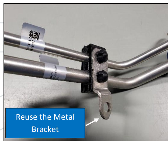
Figure 32: Reuse metal OEM bracket
