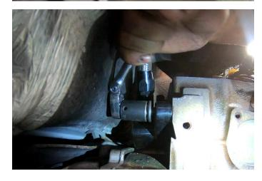
**STEP 18:** With the coolant line routed above the exhaust manifold, thread the available end onto the AN style fitting of the installed thermostat riser block.
