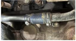
**STEP 8:** Using an 8mm Socket, remove the three bolts anchoring the stock thermostat housing. It is not necessary to remove or disconnect the thermostat housing from the upper radiator hose. Move it to the side, out of the way of the exposed thermostat, to allow for access.
