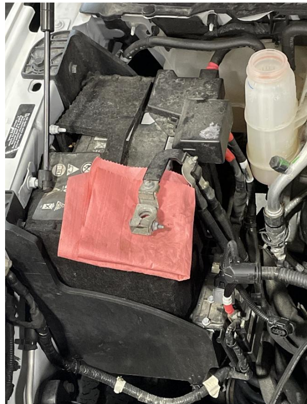
Figure 1: Negative battery terminal disconnected, isolated with a shop rag.
