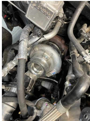
Figure 29: Stock turbocharger, everything removed.
