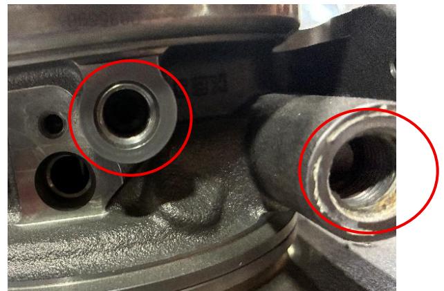
Figure 32: Location for oil feed and coolant feed fitting circled.
