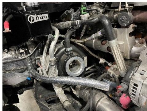
Figure 42: Crankcase Ventilation line and clamp installed onto the CCV fitting.
