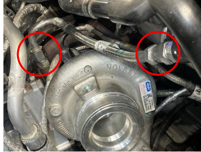
Figure 21: Coolant feed line ends circled.
