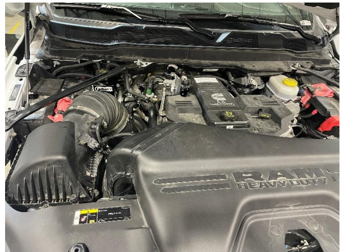
Figure 5: plastic air inlet tube to the right of the air filter housing.
