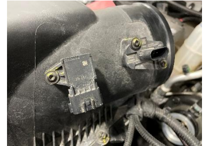
Figure 4B: Barometric pressure sensor and MAF sensor disconnected.
