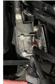
Figure 13: 8MM bolts retaining grid heater relay.
