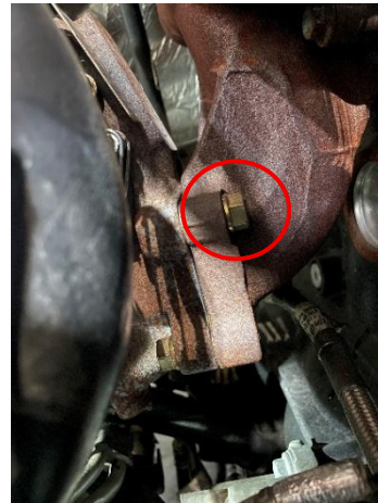
Figure 28: Turbocharger mounting location, mounting nut circled.
