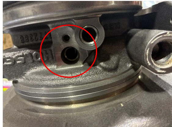
Figure 31: Mounting bore for speed sensor circled.
