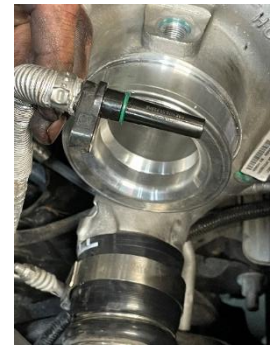
Figure 24B: Turbine shaft speed sensor removed from turbo. Green O-ring seated in its intended location.
