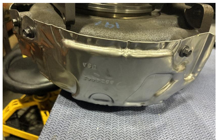
Figure 33: Heatshield on stock turbocharger. Transplant this over to the new Cheetah turbocharger.
