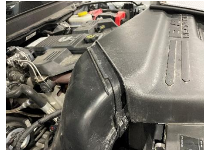
Figure 44: Plastic air inlet tube to the right of the engine air filter housing reinstalled.
