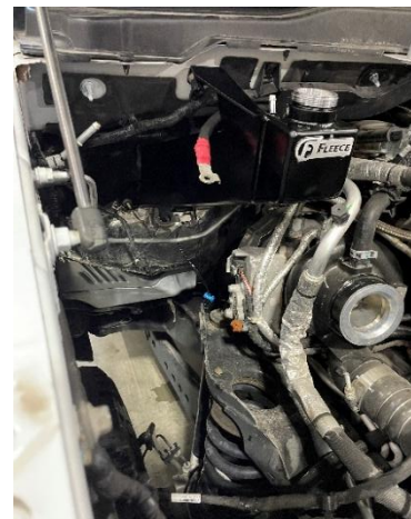
Figure 15: Battery tray removed.
