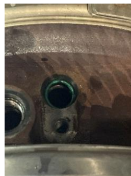
Figure 24A: Turbine shaft speed sensor removed from turbo. Green O-ring intact stuck in mounting bore.
