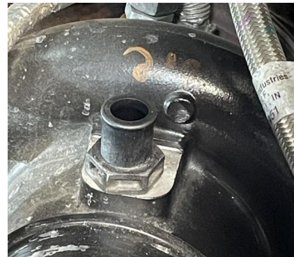
Figure 41: Crankcase Ventilation fitting installed in the new Cheetah turbo.
