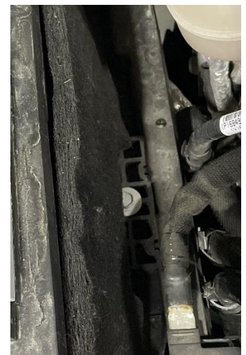
Figure 11: Battery hold down and 10MM retaining bolt.
