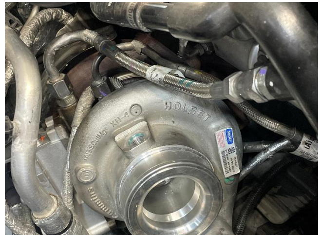
Figure 38: Coolant feed line (top line) and oil feed line (bottom line) reinstalled.
