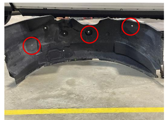
Figure 51: Reinstallation of pushpins for passenger side fender liner.
