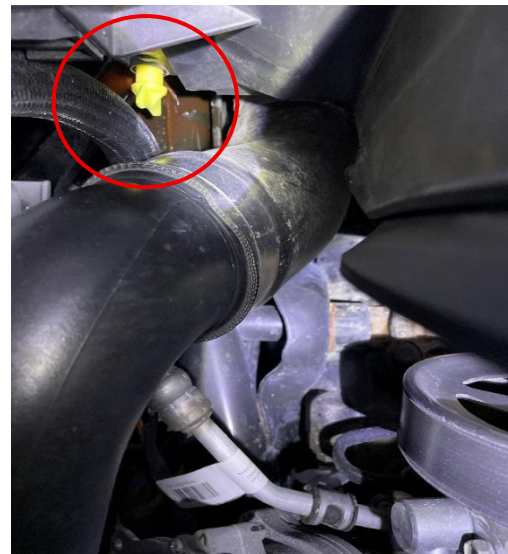
Figure 45: Radiator petcock in open position. Turn clockwise until it is in the closed position.
