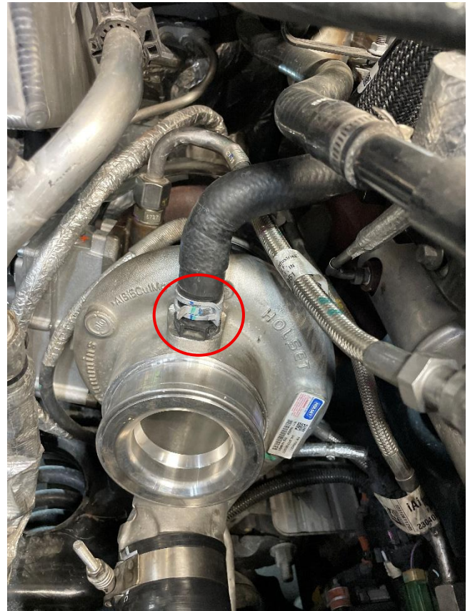
Figure 16: CAC boot and clamp still attached. Crankcase vent hose and clamp circled.
