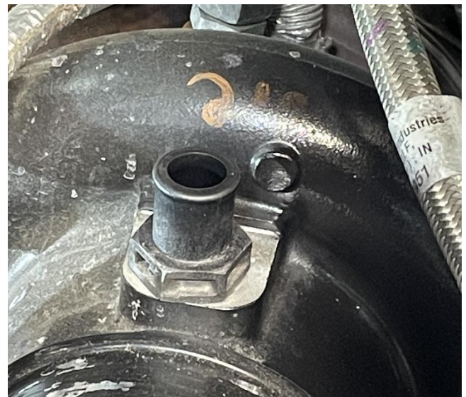
Figure 17: CCV hose and clamp removed. CCV fitting still installed in turbo.
