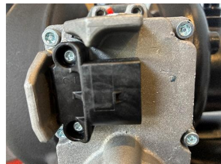
Figure 20: Actuator wiring connector disconnected.
