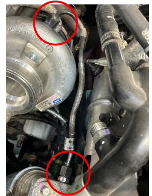
Figure 22: Oil feed line ends circled.
