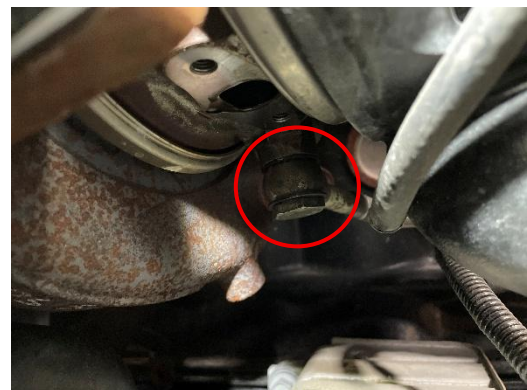
Figure 27: Turbo drain tube removed, coolant banjo line circled.
