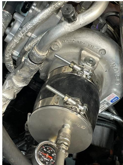
Figure 40: Boost leak tester installed.
