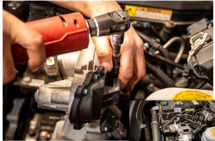
Figure 12: Removal of the four 10MM bolts retaining the EGR Valve. Discard stock gaskets.
