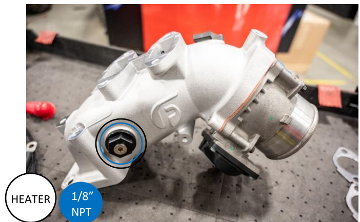
Figure 32: Heater plug and 1/8" NPT installed.
