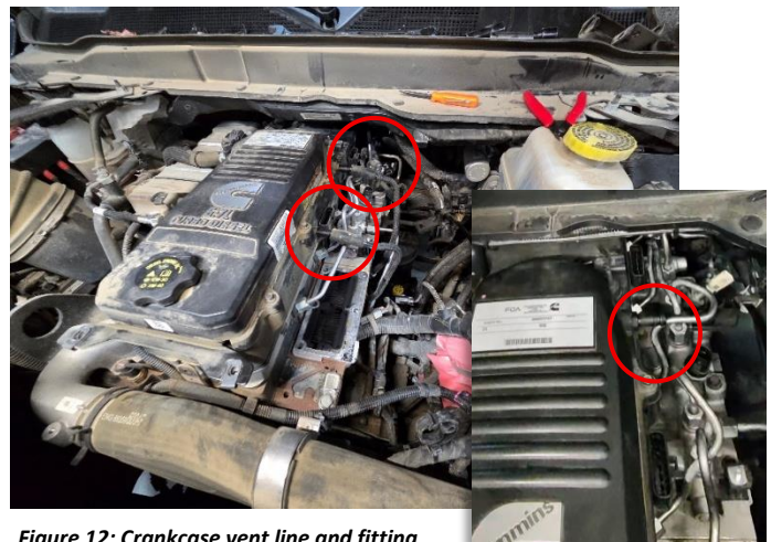
Figure 12: Crankcase vent line and fitting
