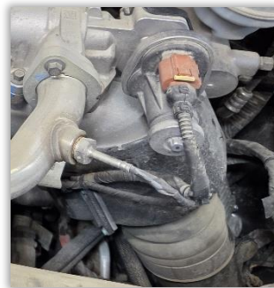
Figure 46: Example image of EGR Valve electrical connector reinstalled.
