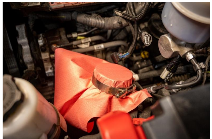
Figure 10: CAC boot covered with shop towel; clamp placed over top to secure.
