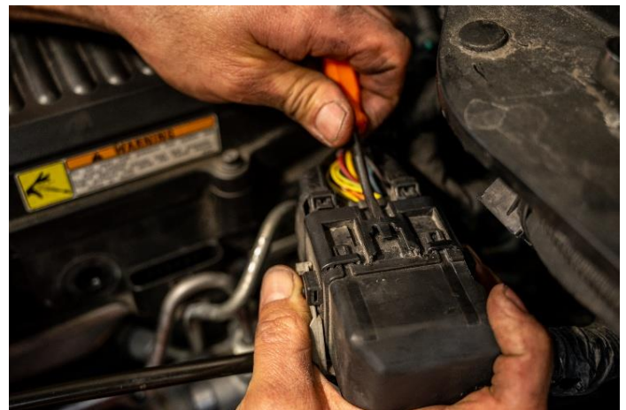
Figure 15: Removal of bulkhead at fire wall.
