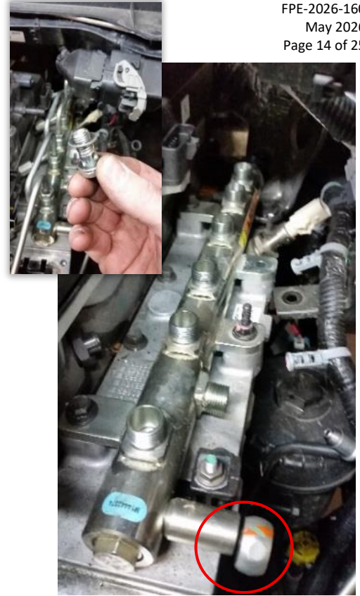
Figure 16: Injection lines removed, fuel return line circled.
