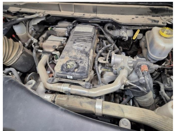
Figure 44: EGR Crossover tube reinstalled Model Years 2019-2024
