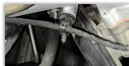
Figure 7B: One of two types of retainers used on harness attached to intake horn. This type is more commonly used in Model Years 2013-2024.
