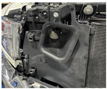
**STEP 30:** Install the grille onto the front of the vehicle. Tighten the two bolts loosened in step 6 using an 8mm socket or wrench. Install the four bolts retaining the top of the grille to the core support using a 10mm socket or wrench.
