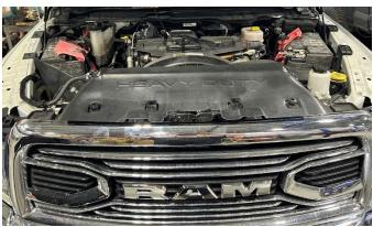
**STEP 32:** Connect the active air connector on the underside of the airbox. Install the airbox into the engine bay. Install the retaining bolt using a 13mm socket or wrench.
