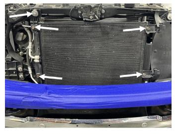
**STEP 11:** Remove the four bolts retaining the power steering cooler using a 10mm socket or wrench. The power steering cooler can be left hanging below the mount to make room for removal of the transmission cooler assembly.
