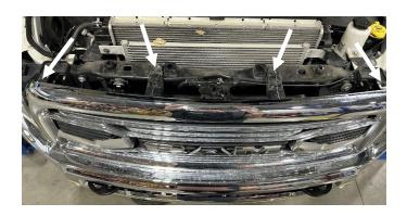
**STEP 7:** Remove the bolt retaining the ram air duct using a 13mm socket or wrench.
