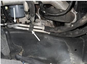
**STEP 17:** Remove the two bolts retaining the transmission lines shown at right using a 13mm socket or wrench.
