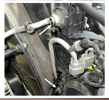
**STEP 15:** Remove the two bolts retaining the passenger side of the OE transmission cooler assembly using a 10mm socket or wrench. Set the bolts aside as they will be reused. Pull the cooler toward the passenger side to remove the inserted mounts on the driver's side. Remove the transmission cooler and attached lines from the vehicle.
