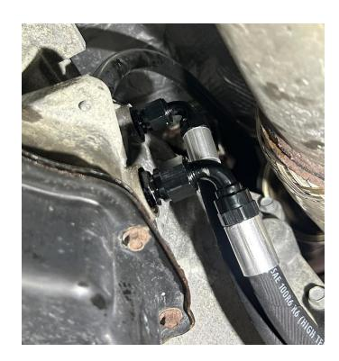
Route the lines under the exhaust pipe, then forward along the frame rail.
