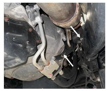
**STEP 18:** Remove the metal retaining clips from both transmission lines on the passenger side of the transmission case using a flathead screwdriver or pick. Place a clean bucket or pail under the transmission to catch any spilled transmission fluid. Disconnect the transmission lines from the transmission.
