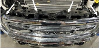
**STEP 31:** Install the upper air dam by clipping the fir tree retainers back into their mounts.
