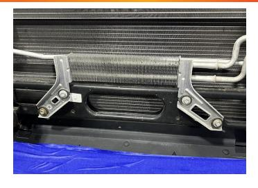
**STEP 12**: Remove the P-clamp retaining the OE transmission cooler line routed to the driver's side of the cooler using a 10mm socket or wrench.
