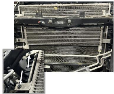
**STEP 16:** Locate the plastic retainer shown at right just inside the passenger fender well and pry the retainer open using a flathead screwdriver or pry tool. Remove the lines from the retainer. Using a 13mm socket or wrench, remove the bolt retaining the clamp to the frame rail a shown at right.
