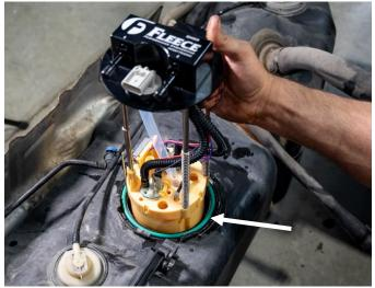
**STEP 14:** Install the locking ring back onto the tank to retain the lift pump assembly. Using a hammer and punch or chisel, turn the ring clockwise until fully seated.
