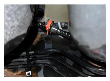
**STEP 5:** Disconnect the red quick disconnect fitting from the fuel filter assembly located on the rear, passenger side of the fuel tank. To disengage the locking tab, spread the two ends of the tab and push the ends toward the center of the fitting. Disconnect the fuel line.
