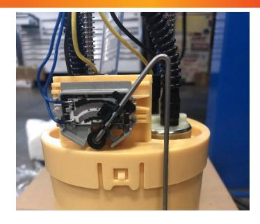
**STEP 13:** Place the included tank flange O-ring onto the tank flange. Carefully install the new PowerFlo lift pump into the tank in the orientation shown at right.
