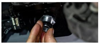
**STEP 9:** Remove the water drain adapter preinstalled on the bottom of the included Donaldson fuel filter. Turn the adapter counterclockwise to remove. Install the included water-in-fuel (WIF) sensor and water drain onto the bottom of the filter. Turn the WIF sensor clockwise until tight.
