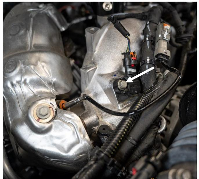
**STEP 3:** Using only a sensor safe cleaner, clean any soot buildup from the MAP sensor.
