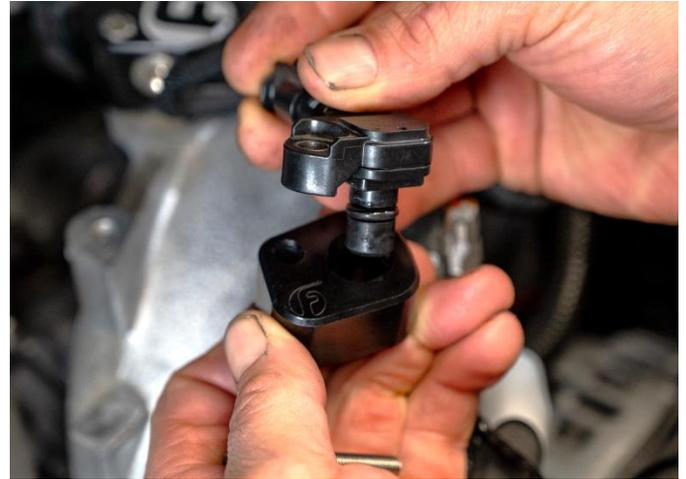
**STEP 5:** Place the included o-ring into the groove on the MAP sensor spacer. Install the spacer into the MAP sensor port on the intake bridge and ensure that the o-ring remains in place.
