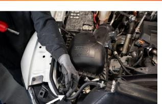
**STEP 8:** Using a 10mm socket or wrench, remove the bolt retaining the battery hold down clamp. Remove the passenger side battery. Using a trim tool, remove the fir trees retaining the solenoid harness to the battery tray.
