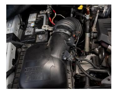
**STEP 29:** Refill the vehicle with coolant and install the OE coolant tank cap onto the Fleece Performance coolant tank.
