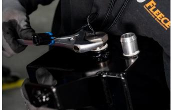
**STEP 19:** Place one of the included SAE size 8 hose clamps onto the OE coolant de-gas line and install the line onto the upward facing hose barb on the Fleece Performance coolant tank. Tighten the hose clamp.
