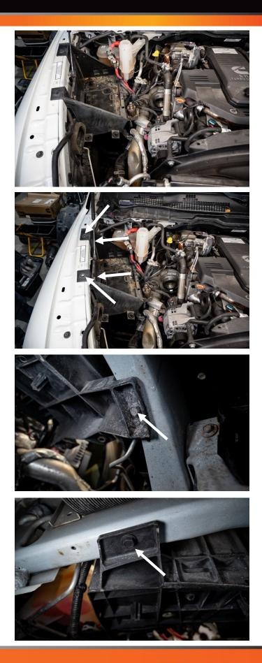
**STEP 10 (optional):** Using a 12mm socket or wrench, remove the nut connecting the main power cable to the battery bus bar. Set the bus bar and harness aside.
