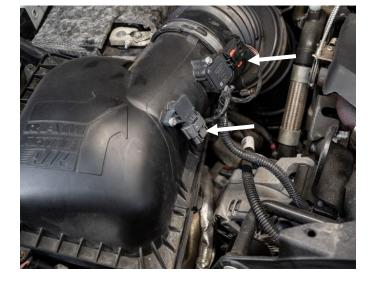
**STEP 5:** Remove the one bolt retaining the airbox assembly to the passenger side fender using a 13mm socket or wrench. Disconnect the active air connector on the lower driver's side of the airbox. Remove the airbox from the vehicle and set aside.
