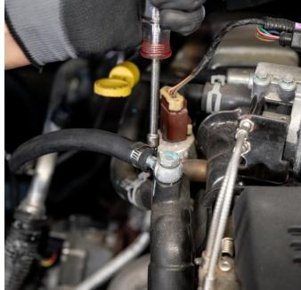
**STEP 21:** Install the included coolant overflow hose (12" cut length) onto the Fleece Performance coolant tank. Route the hose into the fender as shown at right.
