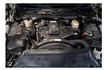
**STEP 3:** Disconnect the mass airflow sensor (MAF) and the barometric pressure sensor. Loosen the hose clamps retaining the intake tube to the upper airbox assembly and the turbocharger.
