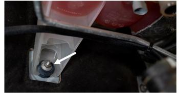
**STEP 16:** Using the included thread sealant, place a thin layer on the threads of the barbed NPT fitting. Install the fitting into the overflow port on the new Fleece Performance coolant tank using an 11mm socket or wrench.
