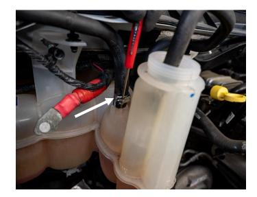
**STEP 13:** Using pliers, loosen the hose clamp retaining the coolant hose to the underside of the OE coolant tank. Disconnect the hose.
