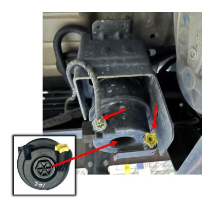
**STEP 4:** Remove the used fuel filter and discard. Remove the green O-ring on the upper fuel filter housing and discard as well.
