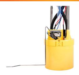
**STEP 11:** Place the included tank flange o-ring onto the tank as shown at right. Insert the PowerFlo unit into the tank in the same orientation as the OE unit.
