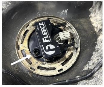
**STEP 14:** Place the fuel tank back under the truck and lift it about six to 8 inches below its normal position. Reconnect the fuel lines and the harness connection. If the vehicle is equipped with a fuel transfer tank, connect the transfer fuel line to the port installed in step 13.
