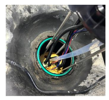
**STEP 12:** Using a hammer and punch/chisel, install the locking ring to retain the PowerFlo unit.
