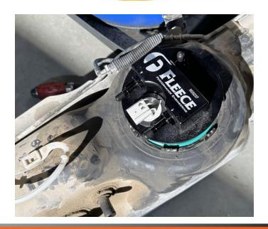
**STEP 26:** Lift the tank about five to six inches below its installed height and reconnect all fuel lines and the electrical connector.
