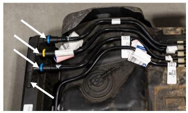
There will be one of two styles of fittings connected to the fuel filter assembly. The fittings can be either blue or yellow in color.
