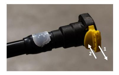
**STYLE #2 – SQUEEZE TAB:** Squeeze the blue tab, then push the fitting towards the filter assembly to disengage the lock. Pull the fitting away to disconnect.
