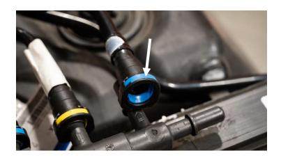
**STEP 7:** With the fuel lines disconnected, push upwards on the fuel filter assembly and remove it from the mount on the fuel tank.
