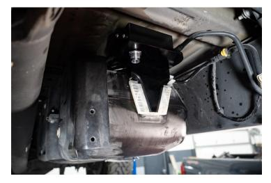
**STEP 9:** Insert the included bolt into the eyelet on the WIF sensor extension harness as shown at right. Install the bolt into the bottom of the mounting notch where the original screw was removed. Using a 10mm socket or wrench, torque the bolt to 10 ft-lbs.
