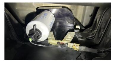
**STEP 13 (SHORT BED VEHICLES ONLY):** Install the guard back onto the tank using the three plastic clips removed in step 3. With the center section of the clip still pulled out, install the clips into the mounting holes. Push the center section into the clip to lock them in place.
