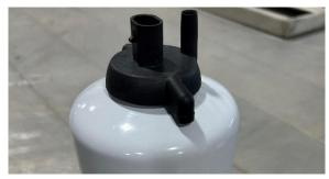
**STEP 12:** Install the included fuel filter onto the filter base. Connect the WIF sensor extension harness to the WIF sensor.
