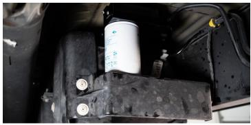
**STEP 14:** Prime the fuel system by cycling the ignition to the on position and waiting five seconds. Repeat this process two to three times, then start the vehicle. Check for leaks.
