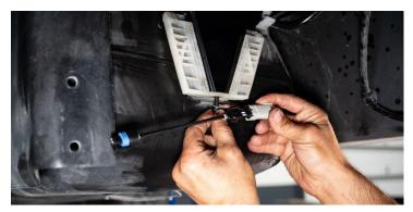
**STEP 10:** Connect the WIF sensor harness to the harness extension.
