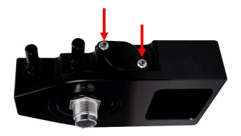
**STEP 3:** Install the fuel heater into the port where the block off plate was removed. Reinstall the screws using a 4mm allen wrench.
