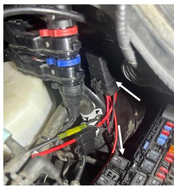
**STEP 5:** Connect the positive and negative battery terminals from the harness onto the driver's side battery. Route the wires as shown at right using zip ties to retain them.
