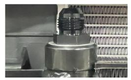
**STEP 13:** Install the 90-degree fitting on the long transmission cooler line onto the passenger side port of the transmission cooler using a 1" wrench. Do not tighten the fitting. Route the line parallel to the top of the transmission cooler assembly.
