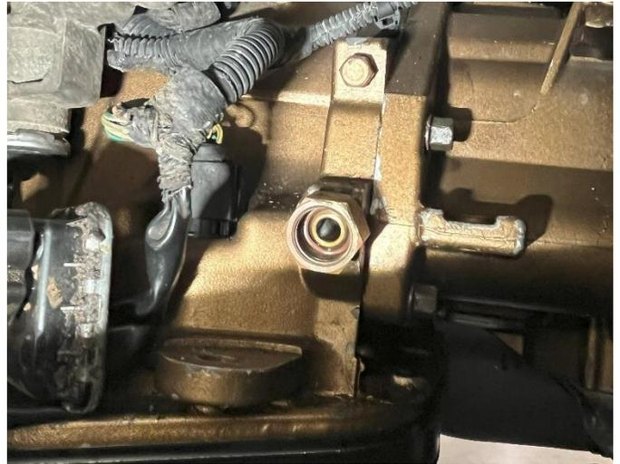
**STEP 10:** Place a bead of thread sealant around the lowest threads and install the two -8AN to 1/4" NPT fittings (item #5) into the transmission ports using a 13/16" wrench. Tighten to 22 ft-lbs. DO NOT OVERTIGHTEN THESE FITTINGS.
