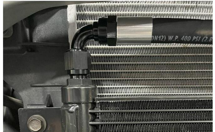
**STEP 14:** Install the 120-degree fitting on the short transmission cooler line onto the driver's side port of the transmission cooler using a 1" wrench. Do not tighten the fitting.
