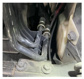
**STEP 6:** Remove the two bolts retaining the transmission cooler. Remove the transmission cooler from the vehicle.
