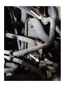
**STEP 9:** Use a 15/16" wrench to remove the two fittings from the transmission.
