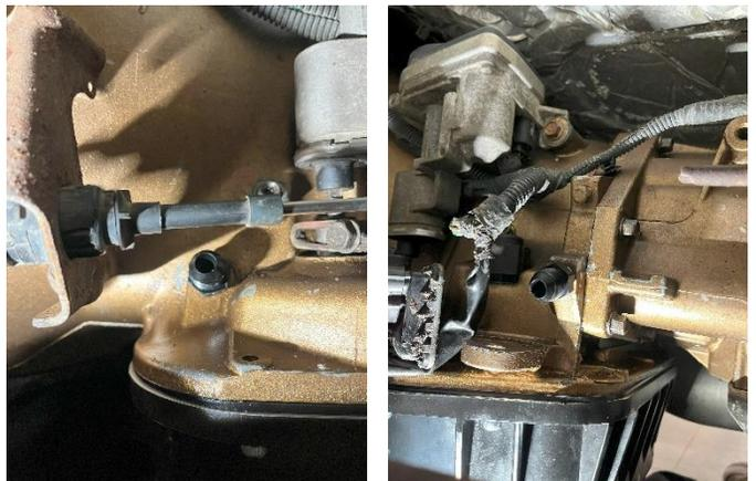
**STEP 11:** Install the new Fleece Performance transmission cooler assembly. Insert the two tabs into the slots, then use a 15mm wrench or socket to install the two bolts retaining the cooler.
