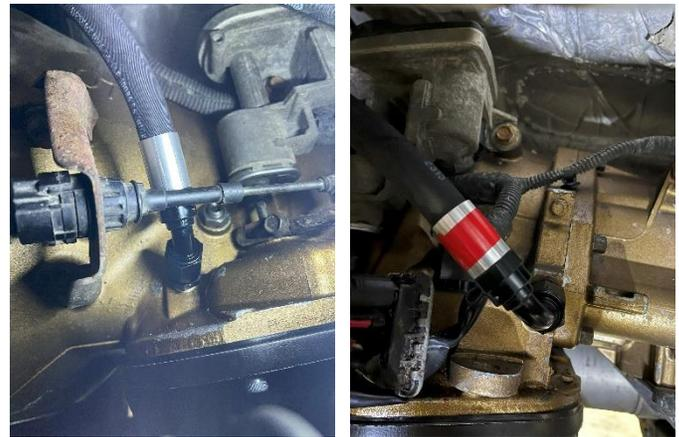
**STEP 17:** Using four double-hose zip ties (item 4), space them evenly along the length of the cooler lines. Tighten the ties to retain the hoses together.
