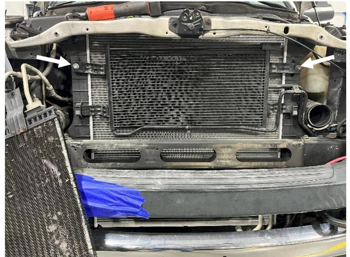
**STEP 7:** Using a 22mm wrench, disconnect both transmission lines from the heat exchanger. Using the included rubber caps, cover the open ports on the heat exchanger.
