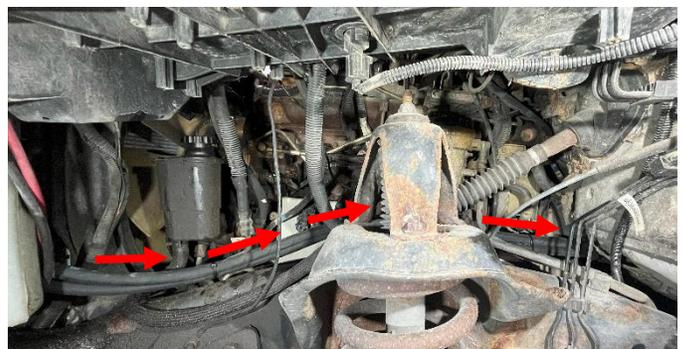
**STEP 16:** Connect the transmission lines to the transmission using a 1" wrench. Do not tighten the fittings. The line routed from the passenger side of the cooler will connect to the front port on the transmission. The line routed from the driver's side of the transmission cooler will connect to the rear port on the transmission. Use a backup wrench when tightening the fittings to prevent overtightening of the AN adapters on the transmission.
