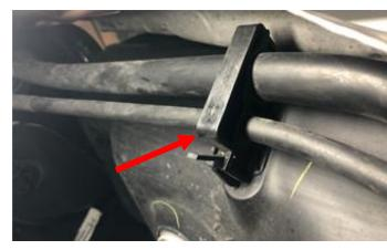
STEP 6: Remove the fuel line quick disconnects. Disconnect the sending unit connector.
