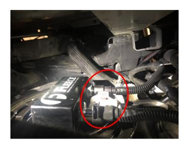
STEP 15: Reinstall your front fuel tank strap. Retain the DEF lines back into the original retention clip. Tighten both tank straps back down.
