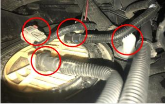
STEP 7: Remove the tank vent located toward the rear of the fuel tank. The vent line is attached to a 3/8'' barb fitting.
