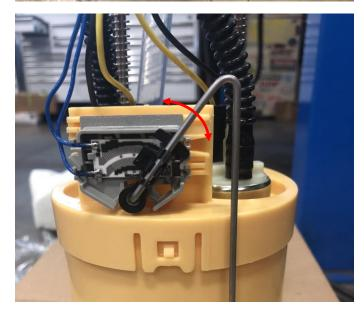
STEP 12: Install the PowerFlo pump assembly into the tank and reinstall the retaining ring using your hammer and punch or chisel by rotating it clockwise to the fully engaged position. Ensure proper orientation of the pump and fittings matches the orientation of the original pump.
