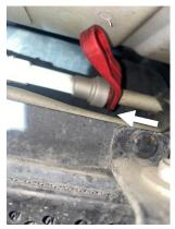
**STEP 5:** Place a transmission jack or floor jack below the fuel tank and lightly support it. Remove the tank straps using a 15mm deep socket. With the tank straps removed, carefully support the fuel tank and lower it down to the ground.
