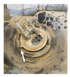
**STEP 10:** Remove the OE sending unit and sealing flange from the tank. Discard the original seal ring.
