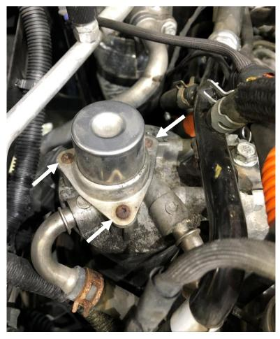
**STEP 2:** Remove all portions of the primer bulb from the top of filter head – these components can be discarded and will not be reused.
