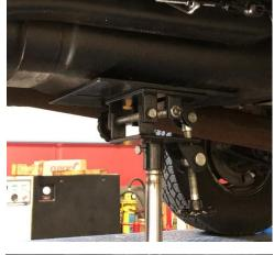
STEP 5: Remove 15 mm nuts that retain the fuel tank straps at the front and rear of the tank. Remove the tank straps.
