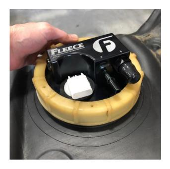
STEP 13: Remove the protective shipping caps from the fittings and install the new fuel line locking tab that is included in your kit onto the return side fitting.
