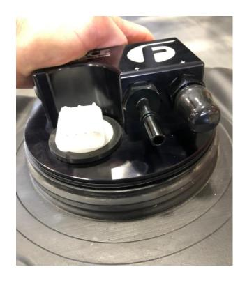
STEP 12: Ensure proper orientation of the PowerFlo by matching the orientation of the original sending unit. Reinstall the retaining ring and tighten using a strap wrench or MATCO tool #FTR730 by rotating it clockwise to the fully engaged position.
