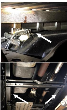
STEP 4: Secure the tank with a lift or jack to lower the tank down to the ground.
