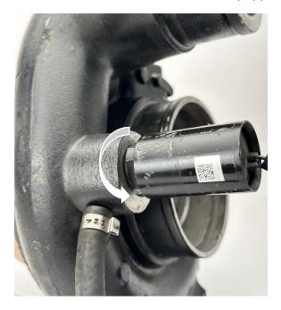
6. Disconnect the exhaust pipe elbow from the turbocharger by loosening and removing the top clamp only. The clamp will be reused.
