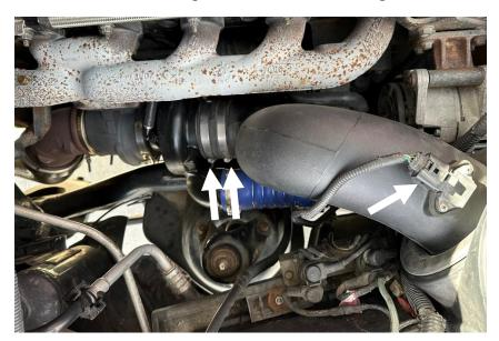
3. Disconnect the turbocharger oil supply line from the top of the turbocharger. Remove the adapter fitting between the oil feed line and turbocharger, this fitting will be reused.
