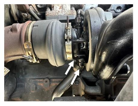
8. Remove the four turbocharger mounting nuts from the manifold and turbocharger. Remove the turbine flange gasket from the exhaust manifold. Discard the original manifold gasket, nuts, and studs.
