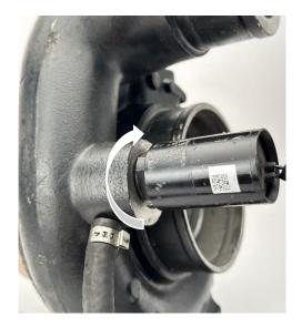
7. Position the intercooler coupler pipe and connect it to the turbocharger. With the clamp in position, tighten the clamp nut to 8 N·m (72 in. lbs.) torque.
