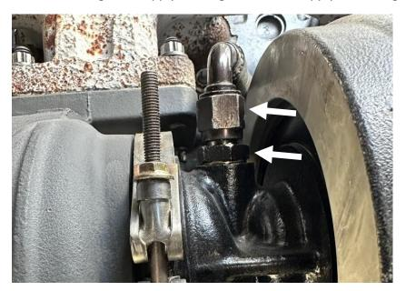
6. For MY 2004.5-2007 trucks equipped with a wastegate control solenoid. Reinstall the solenoid into the front cover of the turbocharger and connect the electrical connector. This instruction only applies to turbocharger model FPE-351-0407.
