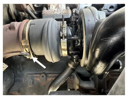
7. Remove the two bolts that retain the turbocharger oil drain tube. Discard the original turbocharger oil drain tube gasket.
