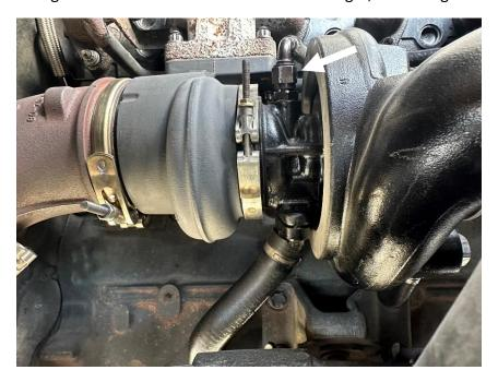
4. Disconnect the intercooler coupler pipe from the turbocharger outlet by loosening and removing the hose clamp. Use caution not to tear the rubber coupler when removing it from the turbocharger. The hose clamp and rubber coupler will be reused.
