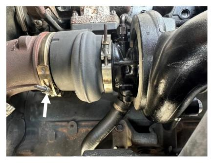
9. Install the air intake tube and re-install the two clamps that connect the intake air tube to the turbocharger. Re-connect the intake air flow sensor connector.
