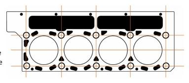
**STEP 4:** Inspect the head stud bores and verify the thread conditions. Clean out any debris using an M14  $\times$  2.0 bottoming tap.
