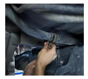
**STEP 5:** Place a transmission jack or floor jack under the fuel tank to lightly support it. Remove the bolts on the tank straps using a 13mm socket or wrench.
