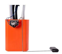
STEP 13: Install the new SureFlo sending unit into the tank. The molded arrow on the fuel tank indicates the location of the alignment tab. DO
