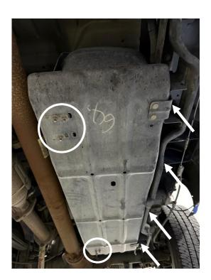
**STEP 5:** Place a transmission jack or floor jack under the fuel tank to lightly support it. Remove the bolts on the tank straps using a 13mm socket or wrench.
