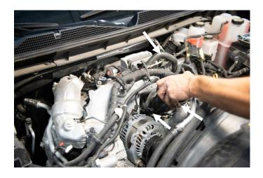
**STEP 8:** Ensure that the square cut o-ring is properly seated into the new Fleece Performance intake horn. Install the new CCV fitting into the intake horn.
