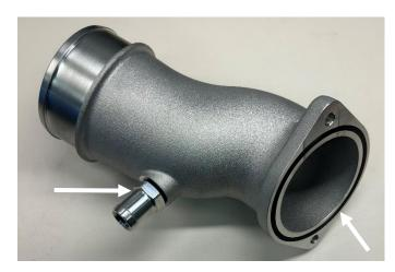
**STEP 9:** Install the new intake horn with the included bolts using a 13mm socket. Be sure that the mating surfaces on the turbocharger and intake horn are clean and free of any contamination before installation. Torque the bolts to 18 ft-lbs.
