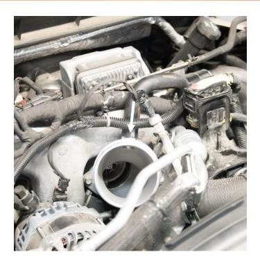
**STEP 13:** Reinstall the intake tube and upper filter housing and connect the mass air flow sensor.
