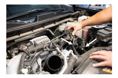
**STEP 4:** Remove the belt from the AC compressor pulley.
