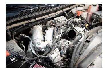
**STEP 3:** Remove the two nuts that retain the AC harness bracket on top of the AC compressor using a 13mm socket. Remove the bracket.
