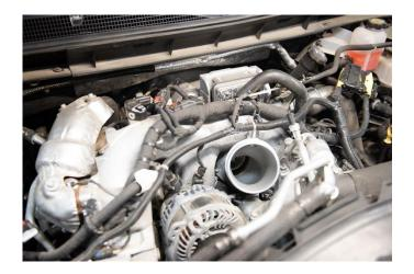
**STEP 12:** Connect the CCV line to the fitting on the new intake horn.
