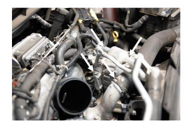
**STEP 6:** Disconnect the CCV hose from the fitting on top of the OE intake horn. Tuck out of the way as shown in the image to the right.
