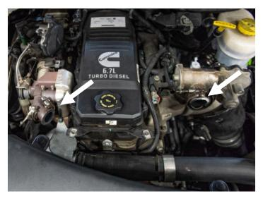
**STEP 16:** Remove the two, 8mm bolts that retain the heat shield to the top of the cooler elbow. Remove the heat shield.
