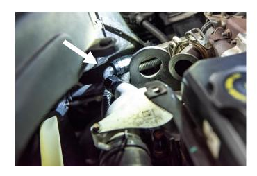
**STEP 22:** Reinstall the heat shield over the coolant bypass elbow.
