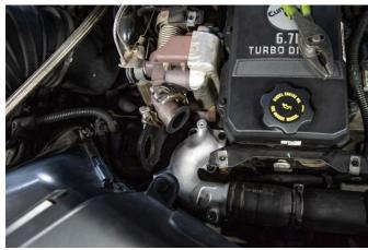
**STEP 21:** Install the coolant bypass hose to the coolant bypass elbow.
