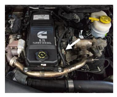
**STEP 13:** Remove the EGR cross over tube.
