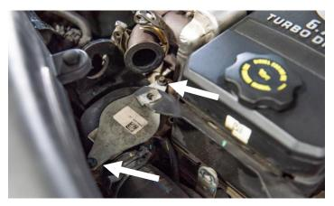
**STEP 17:** Using a pair of channel locks, loosen the clamp that retains the coolant hose to the coolant elbow. Slide it down the coolant hose to allow for removal of the hose from elbow.
