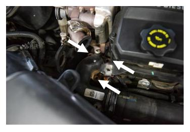
**STEP 19:** Remove the thermostat. Inspect it for wear and proper function. With a Scotch-Brite™ pad and degreasing solution, thoroughly clean the sealing surface of the stock thermostat and thermostat housing. Be sure to remove any foreign debris and reinstall the OE thermostat.
