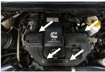
**STEP 12:** Disconnect the EGR temperature sensor connector and retaining clip. There is no need to remove the sensor from the cross over tube.
