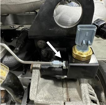
**STEP 28:** Install and connect the back pressure sensor line at both the exhaust manifold and at the sensor block. Torque both flare nuts to 89 in-lbs. Reconnect the exhaust back pressure sensor to the chassis harness.
