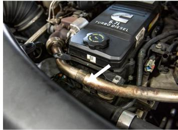
**STEP 15:** Remove the cross over tube and EGR cross over tube gaskets from each end of the tube. Discard the gaskets, new gaskets are provided in the kit.
