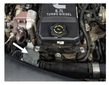
**STEP 23:** Use the double hose clamps provided in the kit to secure the coolant bypass hose to the coolant riser line.
