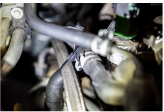
**STEP 24:** Reinstall the EGR cross over tube. Ensure the new gaskets included with the kit are utilized. Install the V-band clamps and the bolt that retains the cross over tube to the front of the engine.
