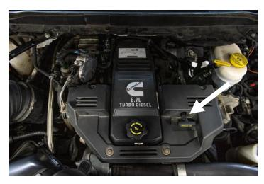
**STEP 11:** Remove the 4, 8 mm bolts that retain the engine shroud and remove the engine shroud.
