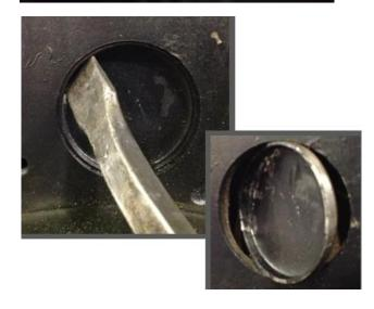
STEP 5: With the freeze plug removed, use a Scotch-Brite™ pad and a degreasing solution to **thoroughly** clean the block surface area from the head down to the rear cover, as well as the bore where the freeze plug was previously installed. Be sure to remove all dirt and foreign debris to allow the coolant bypass thermostat housing to fully seat. If the inner bore where the freeze plug was seated is not thoroughly clean, the O-ring on the coolant bypass housing will not properly seal.
