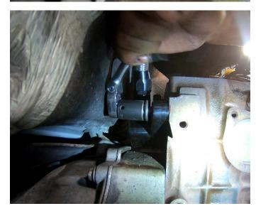
**STEP 10:** Remove the engine oil dipstick.
