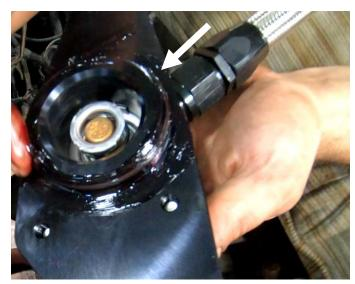
**STEP 8:** Slide the thermostat housing between the firewall and the back of the engine block. Align the thermostat housing with the original freeze plug hole location and press the housing against the engine to seat the housing. The coolant bypass hose should be oriented towards the passenger side of the vehicle.
