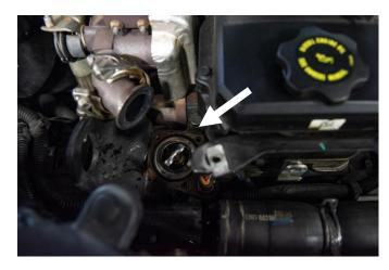
**STEP 20:** Install the new Fleece coolant bypass elbow into the same location as the factory coolant elbow. Install the three new M6 bolts included in the kit that retain the coolant elbow to the cylinder head. Reinstall the coolant hose and clamp.
