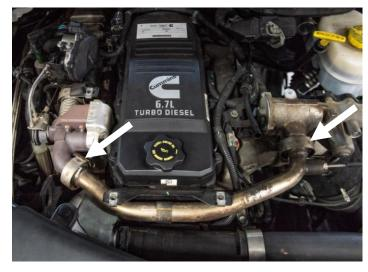
**STEP 14:** Remove the 8 mm bolt that retains the cross over tube at the front of the engine.
