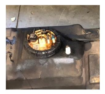
Using a strap wrench, or MATCO tool <u>#FTR730</u>, rotate the sending unit's retaining ring (OE P/N: 52005389) counterclockwise. MATCO tool shown at right for reference. Remove the retaining ring and remove the sending unit assembly from the tank. Have a bucket nearby to catch fuel from the OE sending unit when removed.
