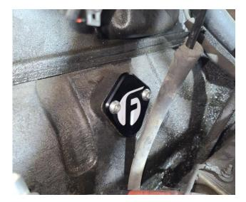
Clean the mechanical fuel pump mounting surface and install the fuel pump block off plate included in the kit.
