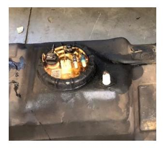
Using a strap wrench, or MATCO tool <u>#FTR730</u>, rotate the sending unit's retaining ring (OE P/N: 52005389) counterclockwise. MATCO tool shown at right for reference. Remove the retaining ring and remove the sending unit assembly from the tank. Have a bucket nearby to catch fuel from the OE unit when removed.
