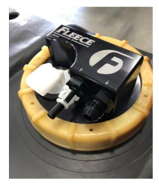
Remove the hex cap to allow for pump return fuel to feed the bucket
