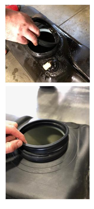
**STEP 10:** Install the fuel level float arm onto the SureFlo sending unit by gently clipping the arm into the fuel level sensor.
