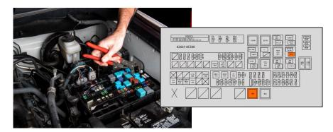
STEP 3: Insert the two relays that were removed through the All Lights On boards with the wire connection facing towards the top of the relay. The board will make a firm connection with the relay.
