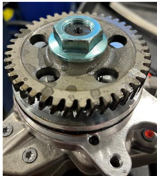
Fig. 2: Install the CP4 nut onto the CP3
