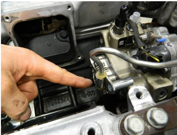
Fig. 3: Carefully remove high pressure line bracket
