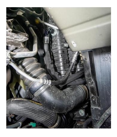
The medium length line is run from the bottom radiator fitting to the "FROM COOLER" port on the transmission. The 45 degree fitting will be pointed slightly inward toward the center of the vehicle and downward
