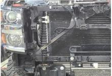
**STEP 6:** To allow for removal of the existing OE lines and installation of the new lines remove the passenger side fender liner.
