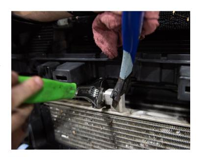
**STEP 11:** Install two of the 7/8"-14 O-ring to - 10AN fittings into the left and right side ports of the oil cooler.
