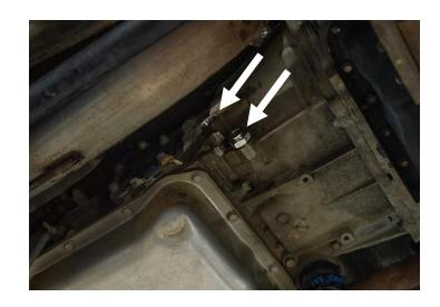
STEP 14: Install two of the 7/8"-14 O-ring to -10AN fittings into the "To Cooler" and "From Cooler" ports on the transmission.
