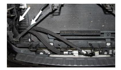
The shortest line is routed from the left side (passenger side) of transmission cooler to the top-side radiator fitting.
