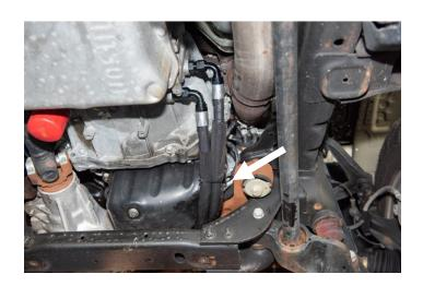
Route the long and medium length lines over the main chassis members and suspension anti-roll bar.
