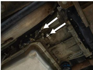
**STEP 9:** With the OE transmission lines removed from the truck, use a 1 1/8" back up wrench and 1 ½" socket or wrench to remove the factory fittings from each side of the transmission cooler.
