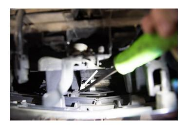
**STEP 5:** Remove the bumper by removing the upper retaining bolts with an 18mm socket.
