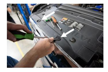
**STEP 3:** Remove the front grill retention bolts located along the top of the grill.
