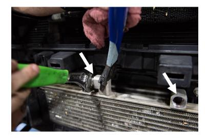
**STEP 13:** Install one of the 7/8"-14 O-ring to -10AN fittings into the passenger-side port of the oil cooler.
