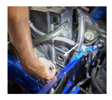
**STEP 16:** Install the two fittings into the radiator, removing and replacing one fitting at a time.
