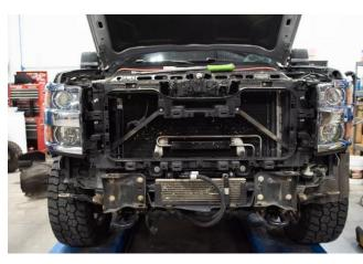
**STEP 9:** Remove the lower engine shroud.
