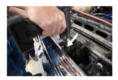
**STEP 4:** Using a long pry bar, release the lower retaining clips for the front grill. Remove the grill.
