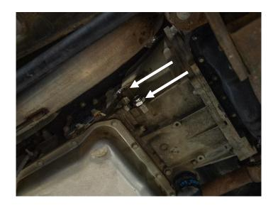
**STEP 12:** With the OE transmission lines removed from the truck, use a  $1 \frac{1}{8}$  back up wrench and  $1 \frac{1}{4}$  socket or wrench to remove the factory fittings from each side of the transmission cooler.
