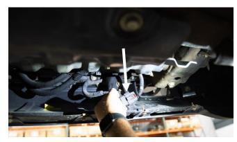
**STEP 7:** Remove the lower supports for the front bumper from the left and right sides of the vehicle.
