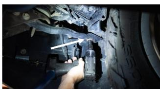
**STEP 8:** Remove the front bumper assembly to provide for clear access to the transmission oil cooler.
