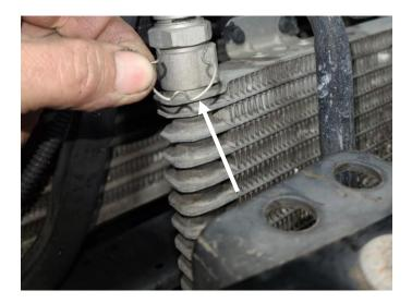
**STEP 11:** With the OE transmission lines removed from the truck, use a 1 1/8" back up wrench and 1 ¼" socket or wrench to remove the factory fittings from each side of the transmission cooler.
