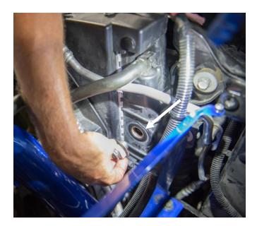
**STEP 14:** Install the two fittings into the radiator, removing and replacing one fitting at a time.
