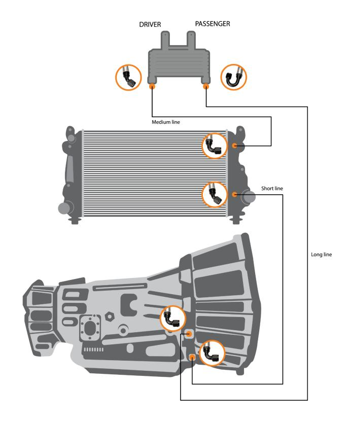
Route the long and short length lines to the transmission closely alongside the transmission bell housing, above the engine oil pan split line. Use zip ties to retain the hose assemblies.
