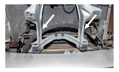
The medium length hose (with the 180-degree fitting) is routed to the left (passenger side) of the transmission cooler. Use the fir tree wire tie to secure the longest hose to the cooler bracket at the hole location shown at right.
