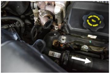
**STEP 18:** Remove the three, 8mm bolts that retain the cooler elbow to the cylinder head. Remove the cooler elbow. The three bolts will be reused for installation of the Fleece coolant bypass elbow.
