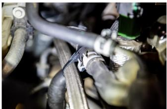
**STEP 25:** Plug in the EGR temp sensor and install the upper engine shroud. Insert the dipstick. Ensure that the coolant drain plug has been reinstalled in the radiator and proceed to re-fill the coolant system. Re-use or replace coolant as necessary to properly fill the system with clean fluid.
