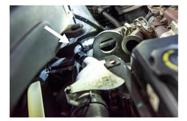
**STEP 22:** Reinstall the heat shield over the coolant bypass elbow.
