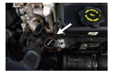
into the same location as the factory coolant elbow. Install the three new M6 bolts included in the kit that retain the coolant elbow to the cylinder head. Reinstall the coolant hose and clamp.
