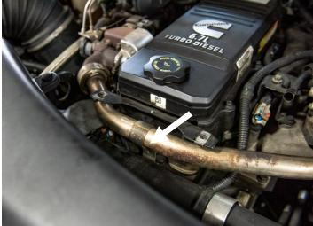
**STEP 15:** Remove the cross over tube and EGR cross over tube gaskets from each end of the tube. Discard the gaskets, new gaskets are provided in the kit.
