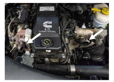
**STEP 16:** Remove the two, 8mm bolts that retain the heat shield to the top of the cooler elbow. Remove the heat shield.
