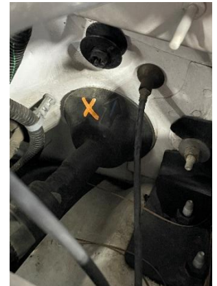
Figure 9: Factory Bulkhead. Incision can be made in rubber boot to route Tapshifter harness.
