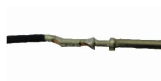
Figure 6: Overdrive Disable pin from (J4) Connector.
