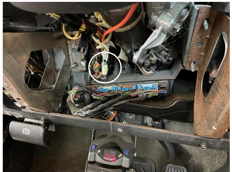
Figure 14: Four pin connector plugged into tapshifter harness. Circled for clarity.
