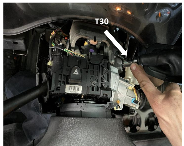
Figure 12: T30 Bolt retaining shift lever, labeled for clarity.
