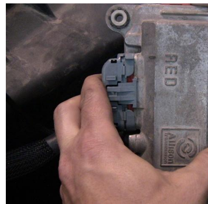
Figure 3: (J4) Connector installed in TCM
