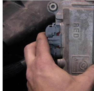
Figure 4: (J4) Connector installed into the red J2 connector on the TCM.
