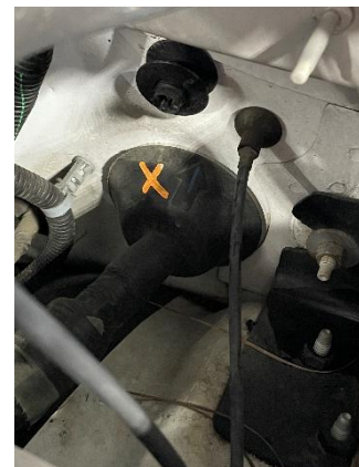
Figure 10: Factory Bulkhead. Incision can be made in rubber boot to route Tapshifter harness.
