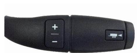
Figure 16: New Tapshifter lever with shifting button, “+” or “-”
