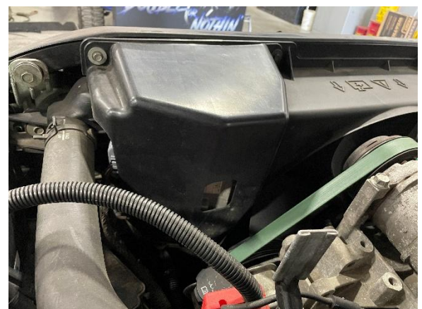
Figure 20: TCM shroud reinstalled.
