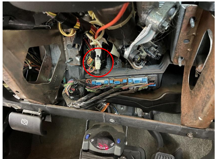
Figure 15: Four pin connector plugged into tapshifter harness. Circled for clarity.
