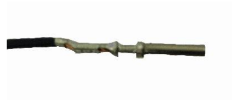
Figure 7: Overdrive Disable pin from (J4) Connector.
