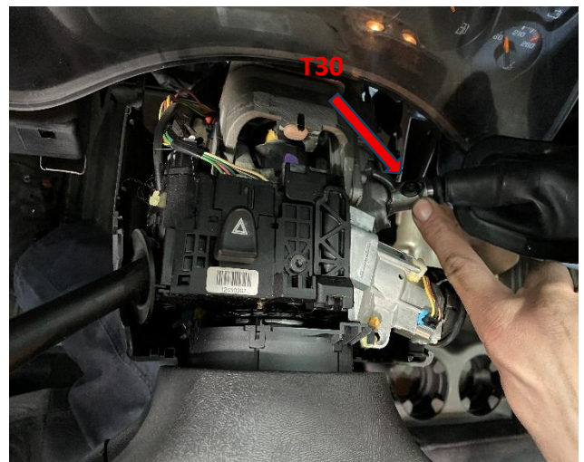
Figure 13: T30 Bolt retaining shift lever, labeled for clarity.
