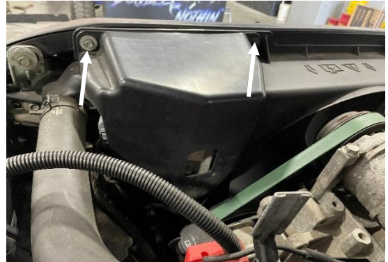
Figure 1: TCM Shroud, retaining bolts highlighted with arrows.
