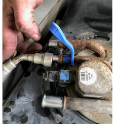
NOTE: Mark the orientation of the sending unit relative to the tank to ensure proper orientation of the SureFlo during installation.
