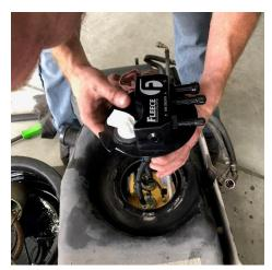
**STEP 12:** Reinstall the original retaining ring using your hammer and punch by rotating it clockwise to the fully engaged position.
