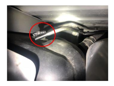
STEP 8: Remove the filler neck hose at the tank with a 9/32" socket to loosen the clamp. Access the clamp through the fender well.
