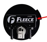
Remove the hex cap to allow for pump return fuel to feed the bucket. MY 2011 and up shown.
