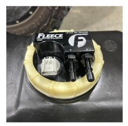
**STEP 13:** Remove the protective shipping caps from the fittings and install the new fuel line locking tabs that are included in your kit onto the return side fitting.
