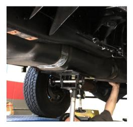
**STEP 7:** With the tank on the ground, make note of the orientation of the OEM sending unit in the tank. The SureFlo sending unit will be oriented in the same manner during installation.
