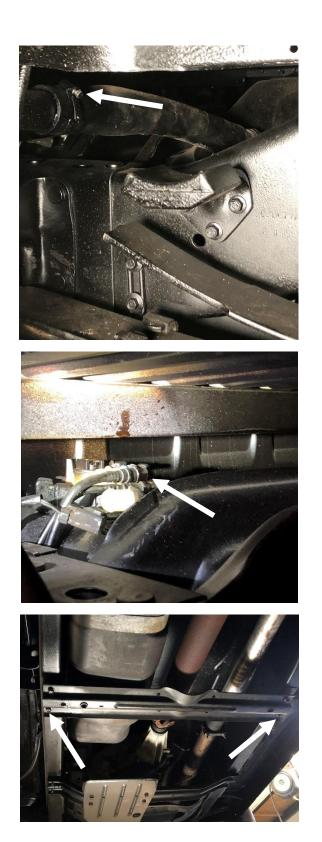
**STEP 4:** Secure the tank with a lift or jack to lower the tank down to the ground.
