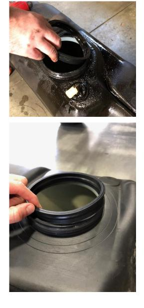
**STEP 10:** Install the fuel level float arm onto the SureFlo sending unit by gently clipping the arm into the fuel level sensor.
