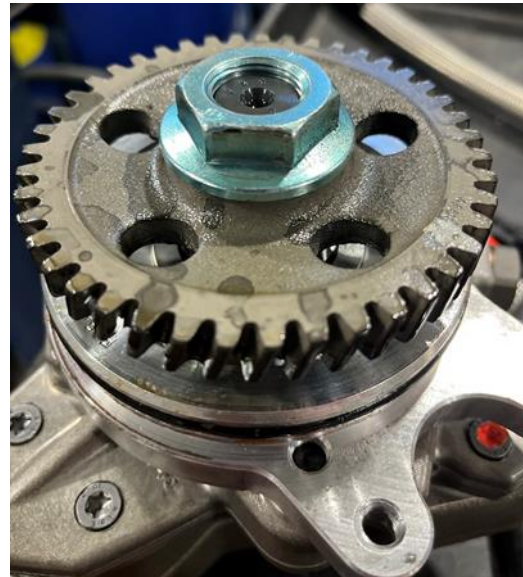
Fig. 12: Install the CP4 nut onto the CP3
