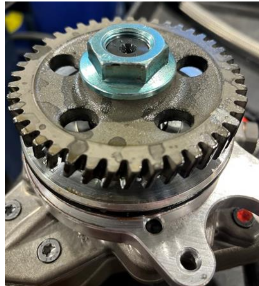
Fig. 12: Install the CP4 nut onto the CP3
