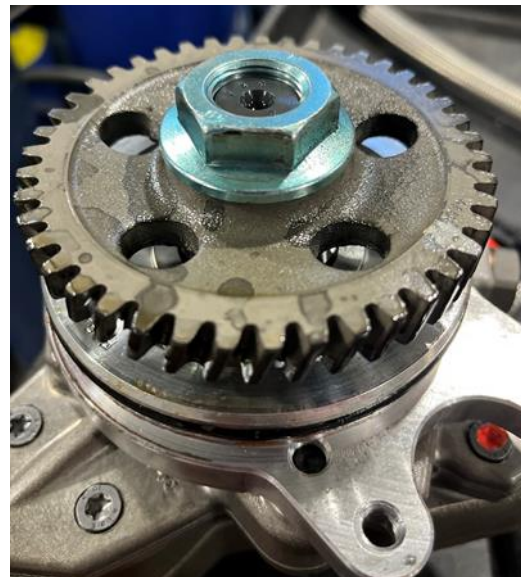
Fig. 12: Install the CP4 nut onto the CP3
