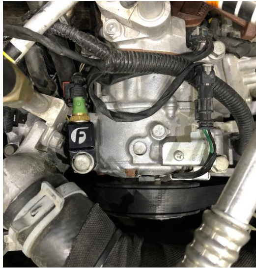
Fig. 18: Fuel temperature sensor block location
