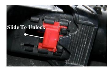
STEP 3: Remove the harness shroud from the TCM connector by gently prying the tabs and separating.
