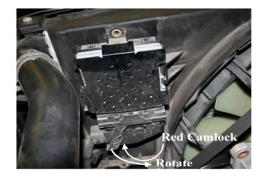
STEP 2: Unhook the TCM harness from the TCM by sliding the red camlock as shown and rotating the camlock lever. Gently pull the connector from the TCM.
