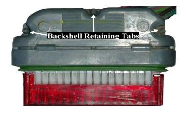
STEP 4: Locate cavity number 29. The wire in cavity 29 controls the Torque Converter Clutch (TCC) and is brown or tan.
