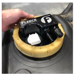
**STEP 13:** Remove the protective shipping caps from the pump cap and install the new fuel line locking tab that is included in your kit onto the return side fitting.
