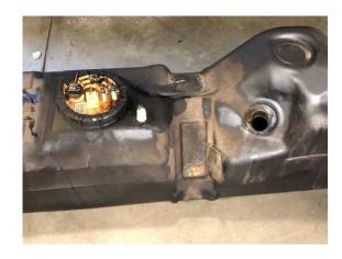
Using a strap wrench, or MATCO tool #FTR730, rotate the sending unit's retaining ring (OE P/N: 52005389) counterclockwise. MATCO tool shown at right for reference. Remove the retaining ring and remove the sending unit assembly from the tank. Have a bucket nearby to catch fuel from the OE sending unit when removed.
