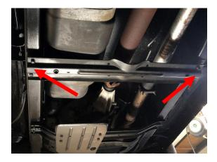
**STEP 4:** Secure the tank with a lift or jack to lower the tank down to the ground on.
