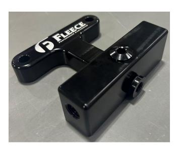
**STEP 30:** Use the bolts removed from the OE fuel bowl to mount and retain the new fuel distribution block as shown at right. Leave the bolts loose as they will be removed and reinstalled upon installation of the fuel filter base.
