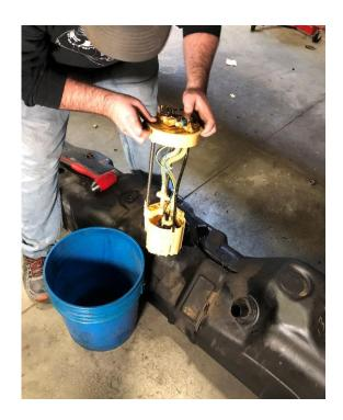
**STEP 8:** Remove the original gasket from the tank.
