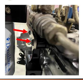
**STEP 34:** Install the included o-ring onto the filter snout on the filter base assembly. Install the WIF sensor onto the fuel filter. Install the filter onto the filter base assembly. Connect the WIF sensor harness to the sensor on the bottom of the fuel filter. Install the o-ring to AN adapters onto the filter base assembly.
