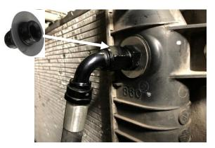
**STEP 2:** Install each of the fittings in the transmission and front mounted auxiliary cooler. Image shown at right is of an LB7/LLY vehicle.
