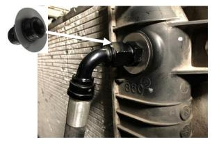
**STEP 2:** Install each of the fittings in the transmission and front mounted auxiliary cooler. Image shown at right is of an LB7/LLY vehicle.
