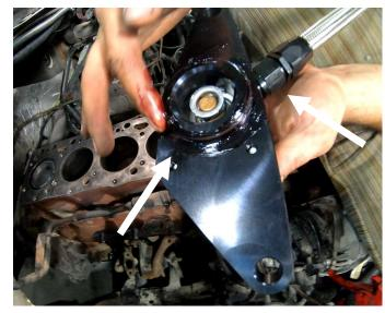
**STEP 10:** Slide the thermostat housing between the firewall and the back of the engine block. Align the thermostat housing with the original freeze plug hole location and press the housing against the engine to seat the housing. The coolant bypass hose should be oriented towards the passenger side of the vehicle and over the exhaust manifold.
