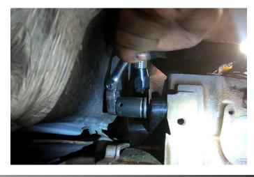
**STEP 12:** Route the coolant bypass hose above the exhaust manifold and thread the hose fitting onto the coolant riser block fitting. Using a backup wrench, tighten the fitting.
