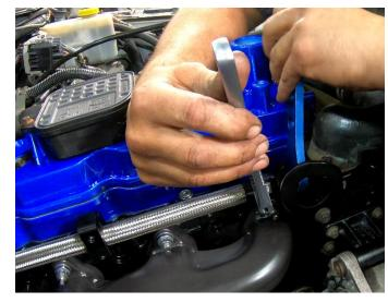
**STEP 13:** Utilizing the coolant bypass hose brackets and M8 socket head cap screws in your kit; position the clamps over the bypass coolant hose and fasten them to the cylinder head in the available tapped holes between cylinder numbers 2 & 3 as well as between cylinder numbers 4 & 5.
