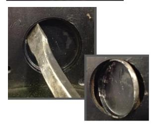
STEP 13: With the freeze plug removed, use a Scotch-Brite ™ pad and a degreasing solution to **thoroughly** clean the block surface area from the head down to the rear cover, as well as the bore where the freeze plug was previously installed. Be sure to remove all dirt and foreign debris to allow the coolant bypass thermostat housing to fully seat.
