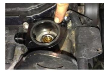
**STEP 11:** Place the stock thermostat housing over the thermostat riser block. Using the supplied M6 flange head bolts, tighten the bolts to 89 in-lbs.
