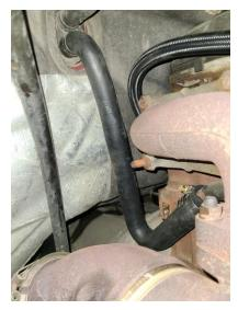
**STEP 8:** Using an 8mm Socket, remove the three bolts anchoring the stock thermostat housing. It is not necessary to remove or disconnect the thermostat housing from the upper radiator hose. Move it to the side, out of the way of the exposed thermostat, to allow for access.
