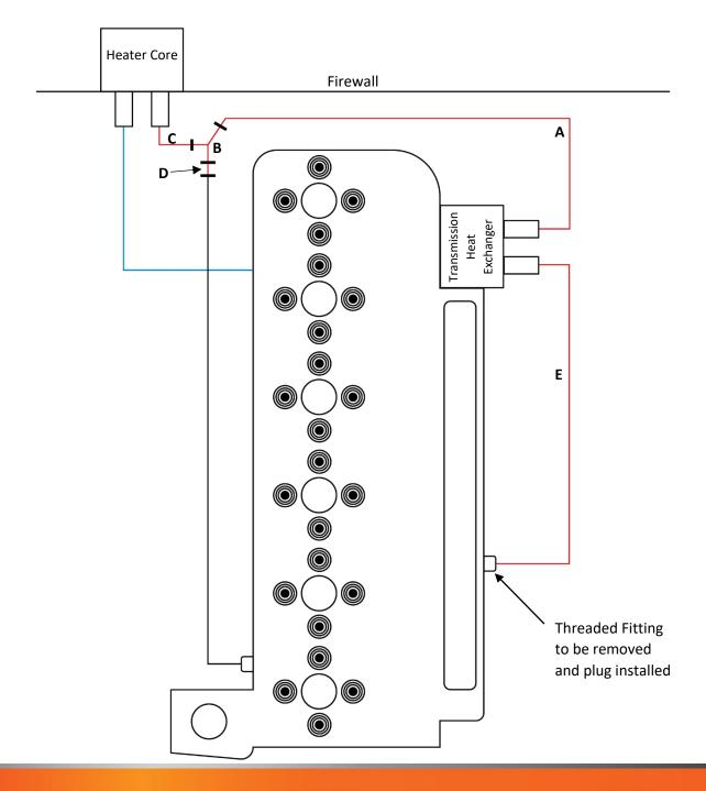
**STEP 5:** Install the rubber caps onto the open ports on the transmission heat exchanger.
