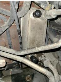
**STEP 6:** Install the 16mm coolant plug port into the engine block where the barb fitting was removed.
