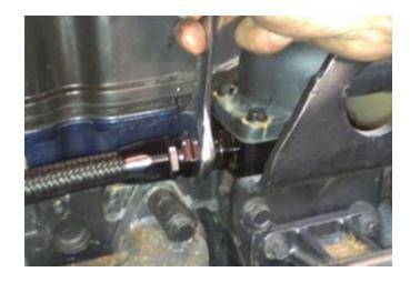
**STEP 19:** Utilizing the coolant bypass line riser brackets and M8 socket head cap screws in your kit; position the clamps over the bypass coolant line and fasten them to the cylinder head in the available tapped holes between cylinder numbers 2 & 3 as well as between cylinder numbers 4 & 5.
